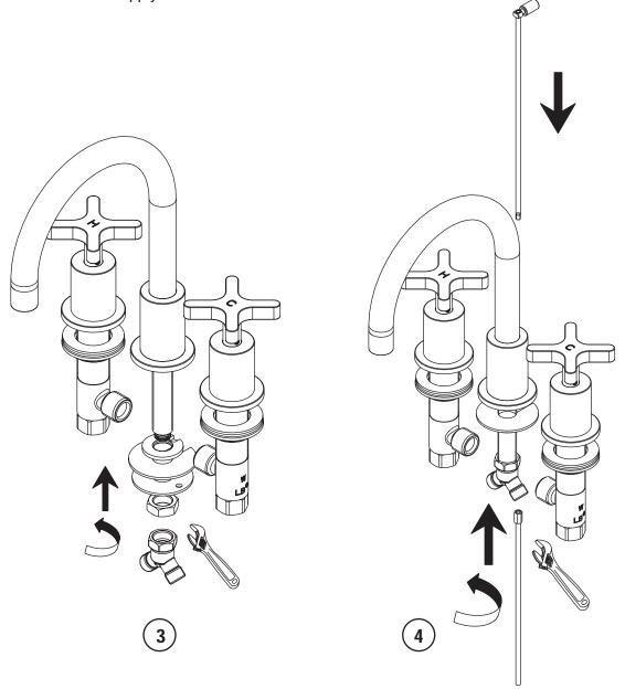
Fit spout and install the connector assembly.
